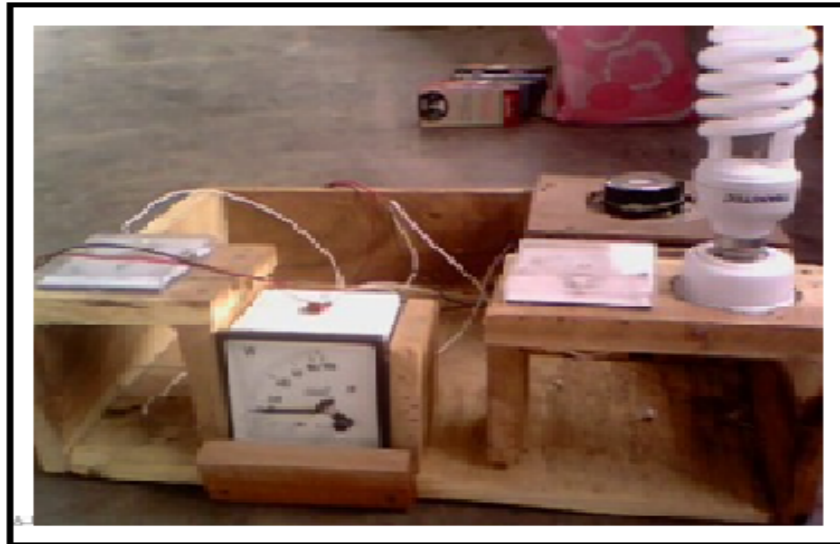
Figure.5: Measurement of power factor with capacitor.
