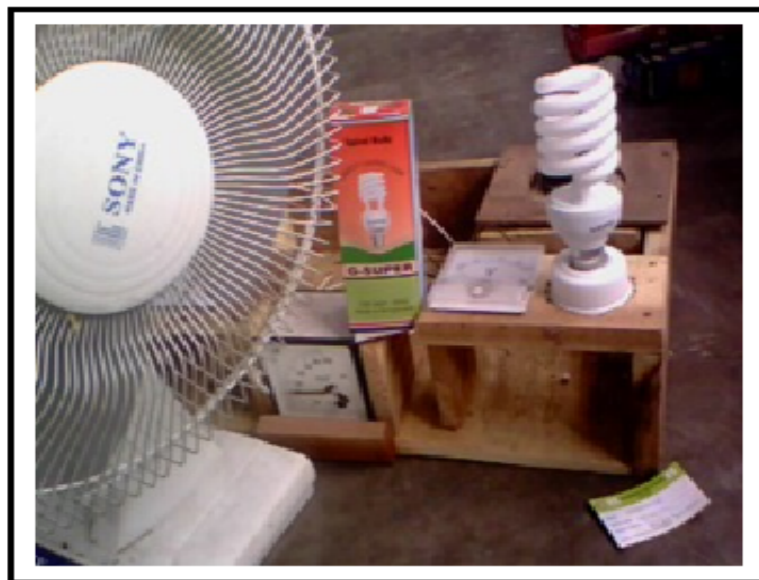
Figure9: Measurement of power factor with inductive load.
