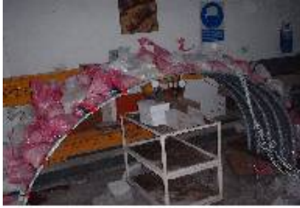
Fig. 7. Sand bag loading on cylindrical shell roofing
